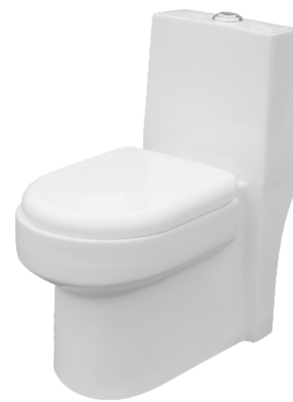
1012 Wash Down L 645 W 360 H 745 mm S - Trap - 225mm (9") P - Trap - 180mm
