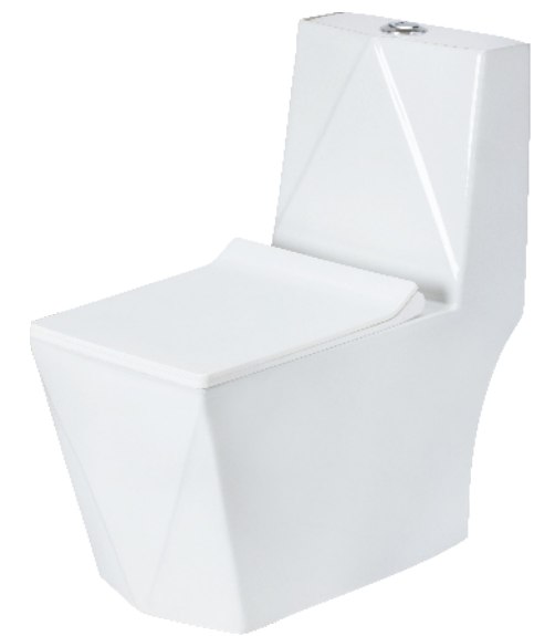
1007 Wash Down L 670 W 375 H 760 mm S - Trap - 225mm (9") P - Trap - 180mm
